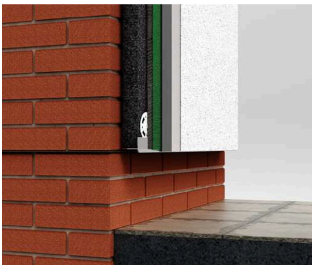
Base bead installed 150mm from ground
