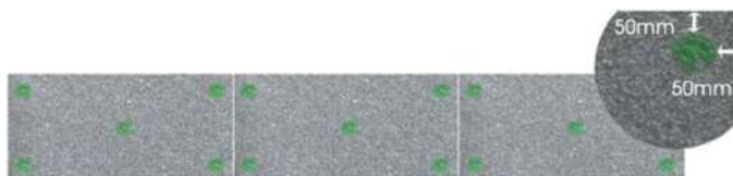
Standard 5 fixings per board
