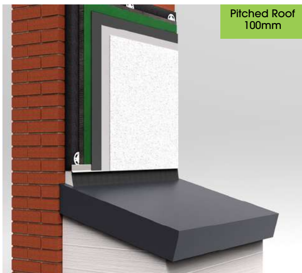
Roof abutment detail leaving a 100mm/ 150mm gap between starter track and roof
