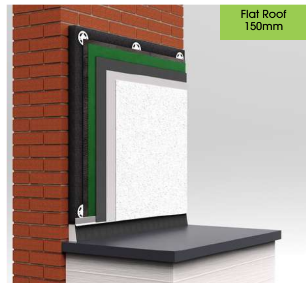
Roof abutment detail leaving a 100mm/ 150mm gap between starter track and roof
