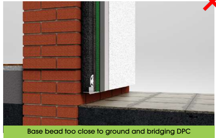
Large cold bridge allowing heat loss and creating potential condensation issues
